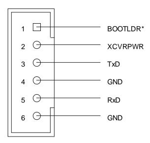
pin 1 – BOOTLDR\*, pin2 – XCVRPWR, and pin 6 – GND are not used in normal applications. pins 3, 4, and 5 provide a 3-wire RS232 connection with no handshaking.
